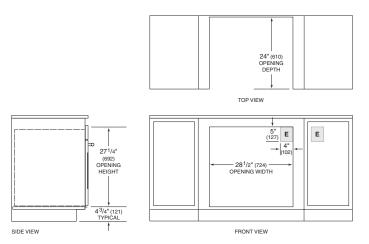
NOTE: Location of electrical supply within opening may require additional cabinet depth. Dashed line represents profile of unit.
